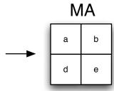
SELECTMB,20,2,2 MOP,LOAD\_BA,4,0,1,3,4 select MB as a 2x2 matrix starting at register 20 copy the 2x2 subset from MA
