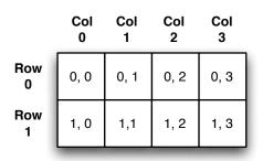
Matrices are stored in sequential 32-bit floating point registers, or in RAM in row major order. The following list shows the storage locations for a matrix of 2 rows and 4 columns starting at register 16.
